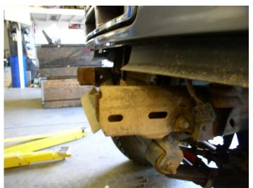
3. Then attach frame mount bracket to bolts coming thru with Flat washers, lock wash-ers and nuts. Don't tighten down you need them to have some adjust-ment.
