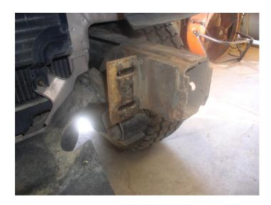
4.Measure distance between brackets and distance between frame. Then adjust the frame bracket to measurement. Then insert frame bracket into frame horn. Use Stock hardware through frame and mounting bracket. You might have to drill the frame horn for throw bolts. You will have up and down and side to side adjustment. Align the bumper to desired
