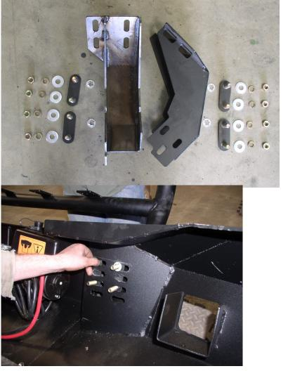
1. Start by Removing Stock Bumper and tow hooks. Install Winch in face of bumper
