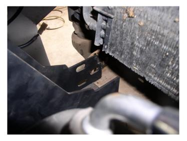
4.Measure distance between brackets and distance between frame. Then adjust the frame bracket to measurement. Then insert frame bracket into frame horn. Use Stock hardware through frame and mounting bracket. Align the bumper to desired adjustment. Tighten up all your bolts.
