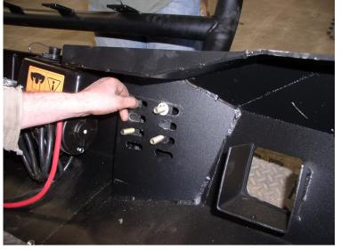
2.Install Double Bolt Plates to the inner bumper mount thru back side wholes provided, securing them with retaining keepers. Then attach frame mount bracket to bolts coming thru with Flat washers, lock wash-ers and nuts. Don't tighten down you need them to have some adjust-ment.
