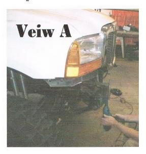
3. Remove Tow Hooks as picture shows View A. After removing them you need to cut the 3 bolt plate from the Tow Hooks as pictured Veiw B flush with the frame. We suggest a chop saw with a metal blade or you can use a torch. Save the 3 bolt plate along with the hardware, they will be used later to secure the frame mount bracket to the frame horn. The Horn will look like this.
