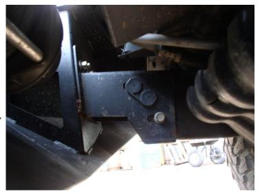
5. We suggest you tack Weld the Frame bracket to the bumper just to make sure it don't come out of adjustment.
