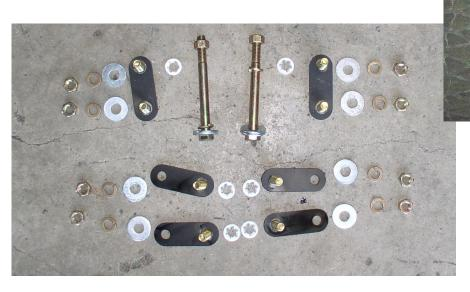
3.Now you install the bolt plate to the bumper mount using the keepers and a socket coming through the back side of the bumper mount push the keeper over the bolt repeat for all other bolt plates See View B
