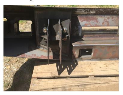
3. Then attach frame mount bracket to driver side bolts coming thru with Flat washers, lock wash-ers and nuts. Don't tighten down you need them to have some adjust-ment.
