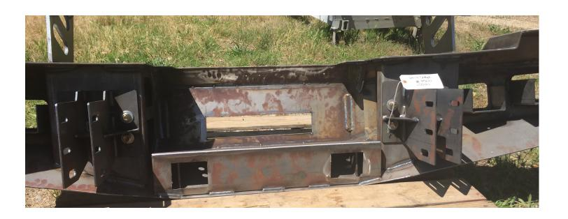
5..Measure distance between brackets and distance between frame. Then adjust the frame bracket to measurement. Then insert frame bracket into frame horn. Use Stock hardware through frame and mounting bracket. Align the bumper to desired adjustment. Tighten up all your bolts.
