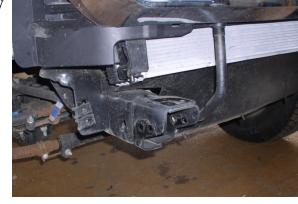
2. Now you will prep the Tow hook cut the hook off with a cut wheel saving the 3 bolt plate. See View A
